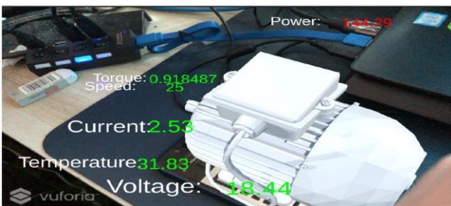
Fig. 5. Values and Motor being displayed in AR to show text tracking
