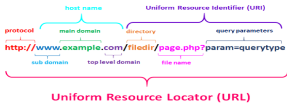
Fig. 1. Uniform Resource Locator Structure (Shivangi et al., 2018)
