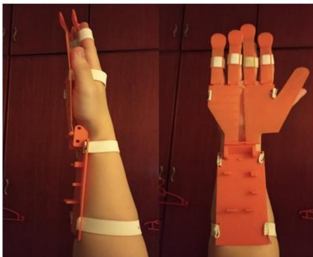
Fig. 7. Mechanical glove fitted with elastic straps.
