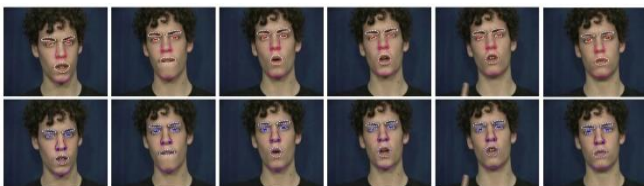
Fig. 11. Shown here is an example of accurate and detailed face detection in each of the frames over a video sequence of an ASL sentence. The top row shows the automatic detection obtained with the algorithm. The bottom row provides a manual detection for comparison. (Ding and Martinez, 2008)
