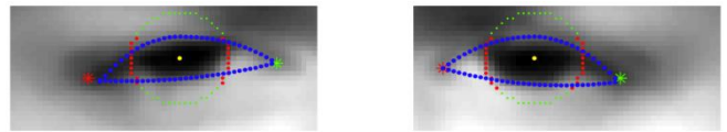
Fig. 12. Eye corners are represented with an asterisk. The iris is shown as a circle, of which, the red part is the visible component. The upper and lower contours of the shape of the eye are shown in blue. (Ding and Martinez, 2008)
