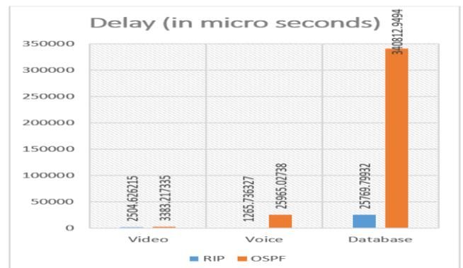
Fig. 12. Delay time Graph RIP vs OSPF
