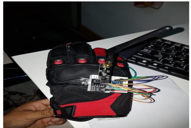
Fig. 8. Hand Glove with NRF24101 and Accelerometer
